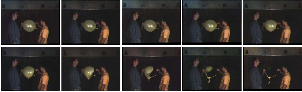
Figure 9: 1560fps video of a popping balloon with rolling shutter distortions. The balloon is struck at the top by the tack, but it appears to pop from the bottom. The top of the balloon seems to disappear.
