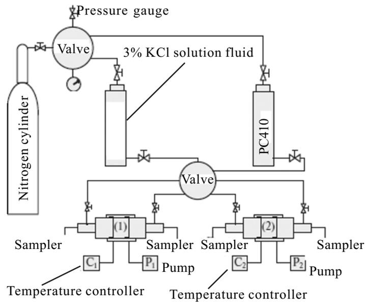
Fig. 1. Experimental plant for studying hydraulic fracturing with self-diverting fluid.
