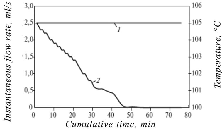
Fig. 5. Results of a filtration test in a filter press: 1 – temperature; 2 – instantaneous flow rate of diverted fracturing fluid.
