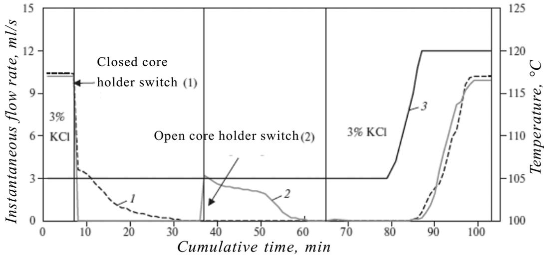
Fig. 4. Results of a study of diversion capacity: 1, 2 – cores with fractures (core 1, core 2); 3 – temperature in core holder.
