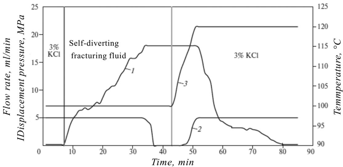
Fig. 3. Results of temporary plugging of self-diverting fracturing fluid. 1 – displacement pressure; 2 – flow rate; 3 – temperature in core holder.
