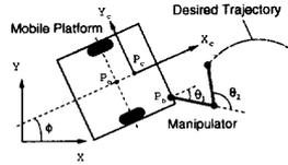
Fig. 1. Schematic of the mobile manipulator.
