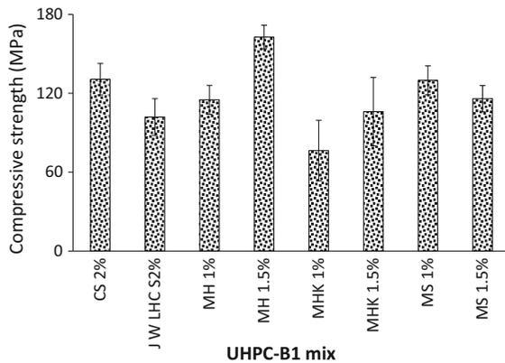
**Fig. 5** Compressive strength test results (UHPC in preliminary laboratory studies (means and standard errors))
