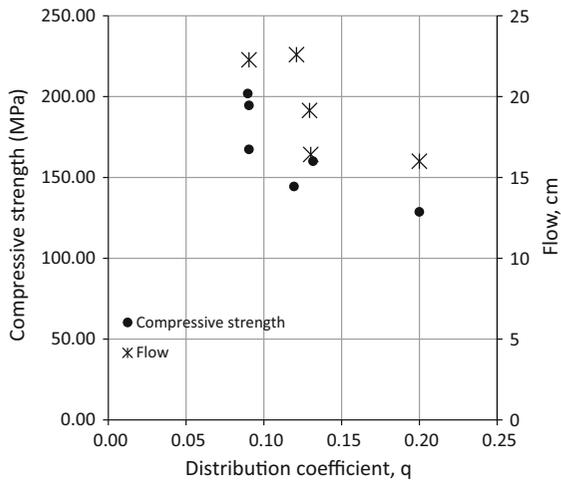
**Fig. 6** Correlations of the distribution coefficient  $q$  with the fresh mix workability (flow) and the compressive strength of UHPC
