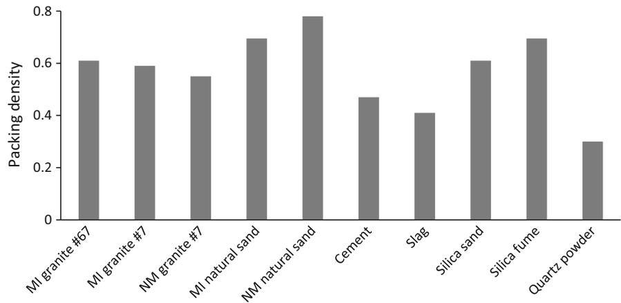
was provided by AGSCO Corporation, Illinois. Size distributions were assessed by sieve analysis, or provided by manufactures. The packing density of each particulate constituent was measured by weighing a 1-l container filled with the particles consolidated on a vibrating table over 2 min. Packing density of different particulate constituent presented in Fig. 1.
