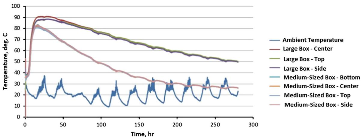
**Fig. 7** Temperature time histories at different locations within the large and medium-sized blocks made with the UHPC prepared at pilot scale
