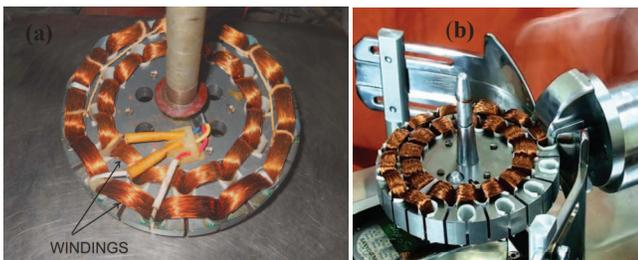
Fig. 7. (a) 24 slot ceiling fan stator (b) In-slot winding machine [9].
