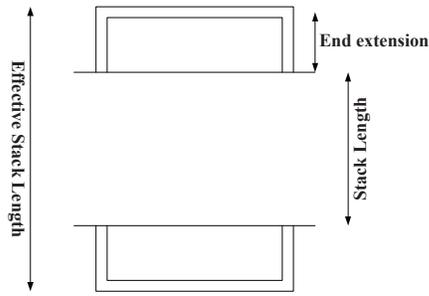
Fig. 8. Effective stack length of a stator.
