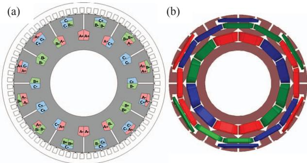
Fig. 6 (a) Dual slot layer 24 slot 10 pole stator and (b) its end connections.
