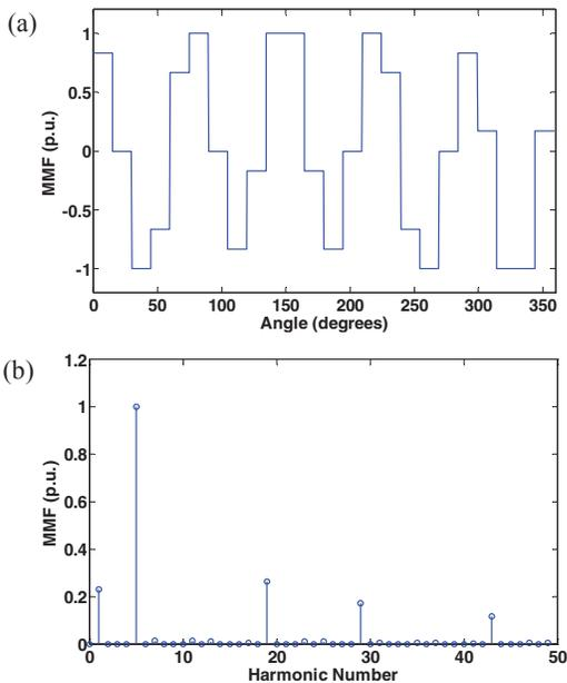
Fig. 2. (a) Air gap MMF of 24 slot 10 pole winding with uniform turns per coil and, (b) its frequency components.
