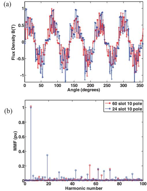
Fig. 10. (a) Air gap flux density of the FSCW and distributed winding designs from FEA and, (b) their frequency components.
