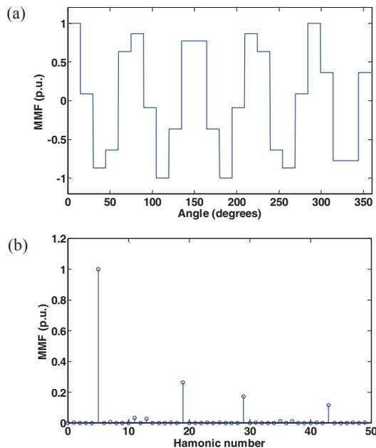
Fig. 5. (a) Air gap MMF of 24 slot 10 pole winding with varying turns per coil and (b) its frequency components.
