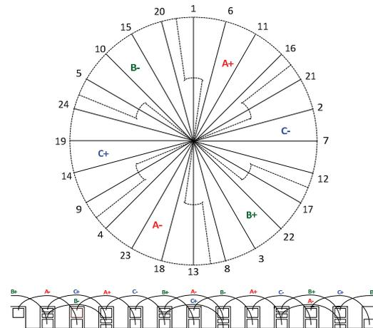
Fig. 1. Star of slots for 24 slot 10 pole multi-layer configuration with uniform turns per coil.
