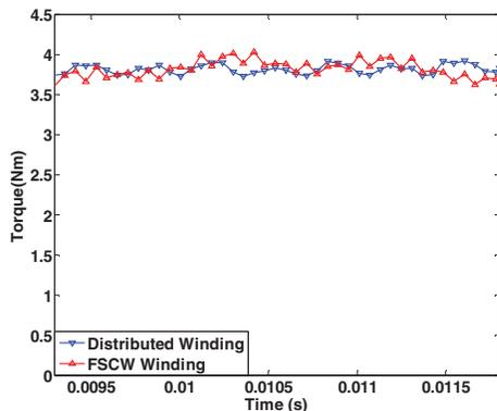
Fig. 12. Instantaneous torque of the FSCW and distributed winding motors at rated slip.
