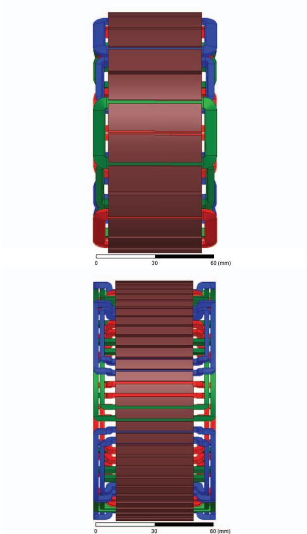
Fig. 9. Comparison of stack lengths of FSCW and distributed winding for the same effective stack length.
