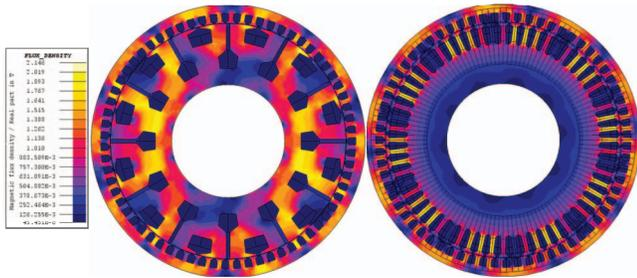
Fig. 11. Comparison of flux density distribution in the FSCW and distributed winding motors.
