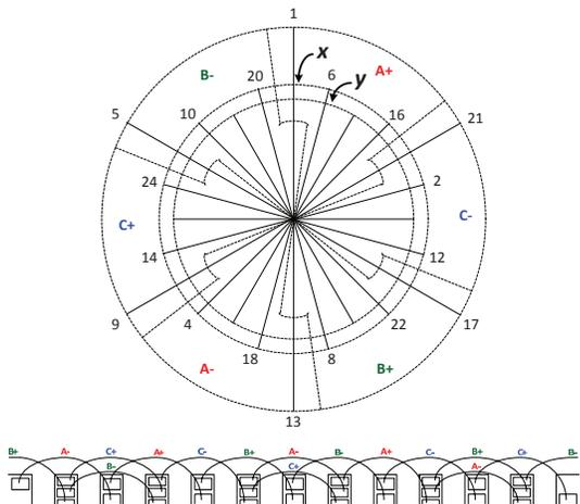
Fig. 3. Star of slots for 24 slot 10 pole multi-layer configuration with varying turns per coil.
