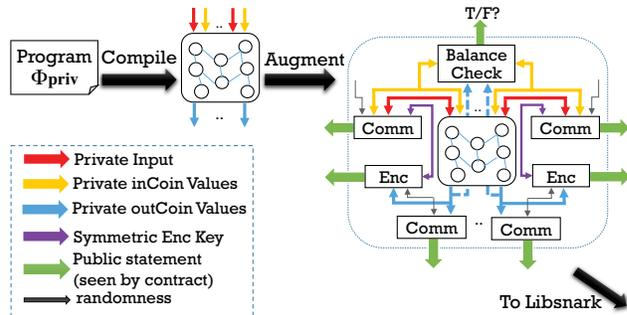
Fig. 7. Compiler overview. Circuit augmentation for finalize.
